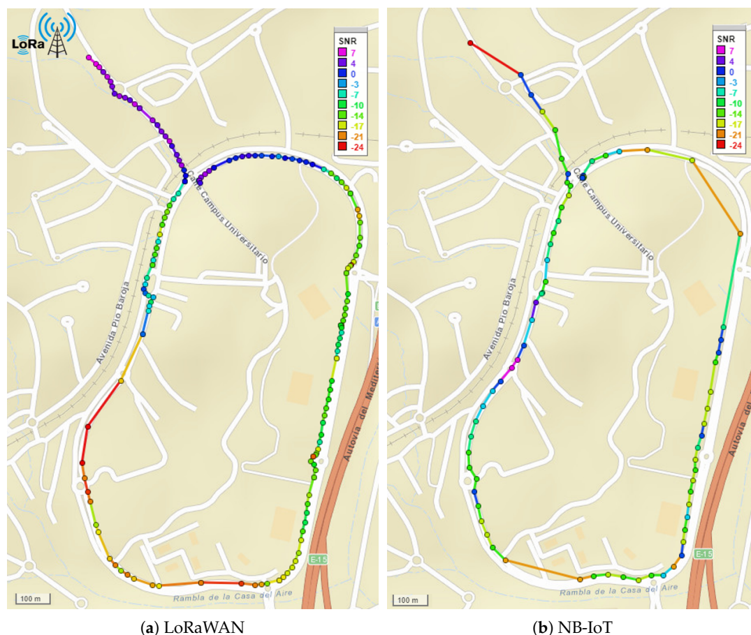
Figure 6. SNR obtained in one test ride around the campus ring.
