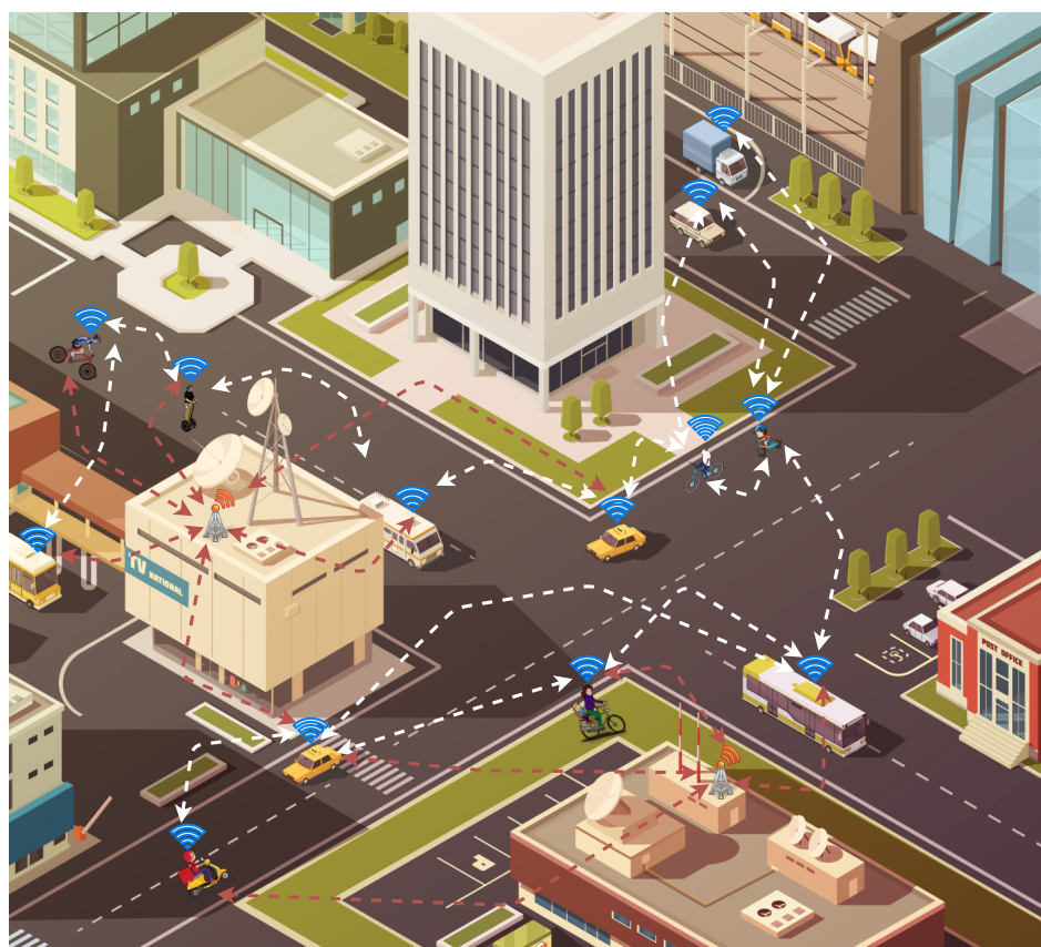
Figure 1. Urban fully-connected vehicular scenario. White/red arrows: V2V/V2I links.
