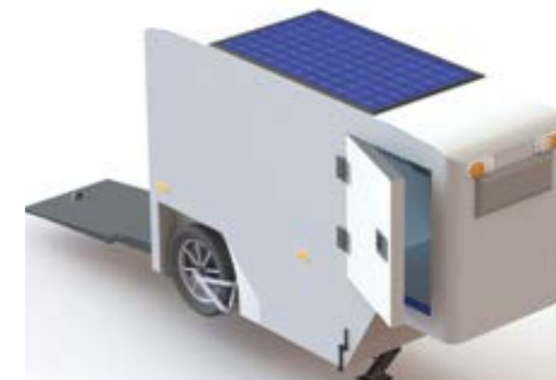
Figure 4.10: Model of the improved fridge-freezer trailer.
