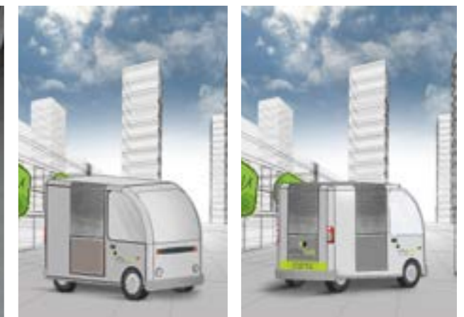
Image 4.4: Concept design for City Hub with space for three to four roll cages.
