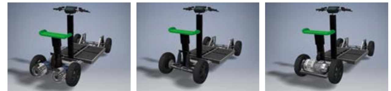
Figure 4.8: Packaging of the drive mechanism with sequential transaxles, in-wheel motors and dual drive.
