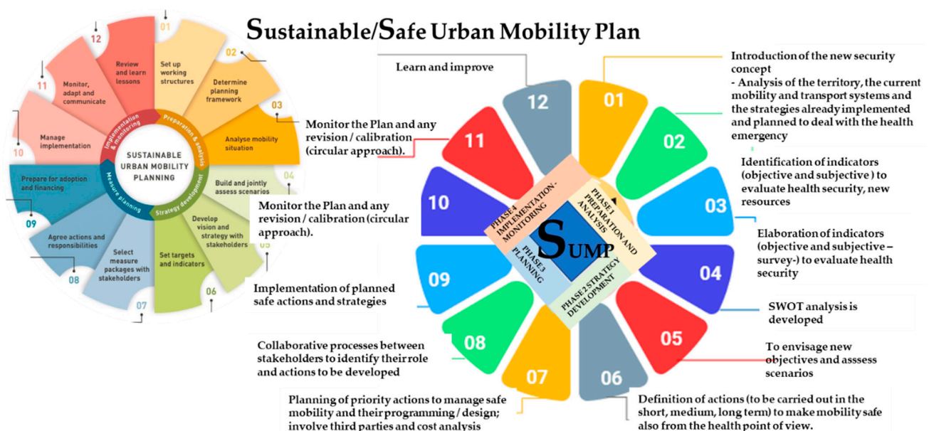
Figure 2. The 12 Steps of Sustainable Urban Mobility Plan (SUMP) and the new circular approach of the Sustainable and Safe Urban Mobility Plan.
