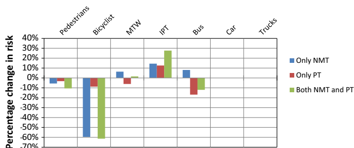
Fig. 8. Percentage change in risk to different road users under three scenarios – Vizag.
